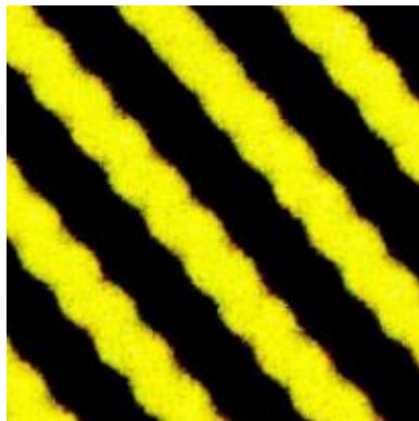
Fig.1. The modulated domain structure of iron garnet film.
